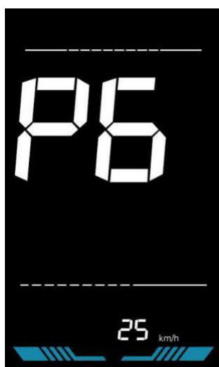
Figure 6-6 Speed limit setting interface
