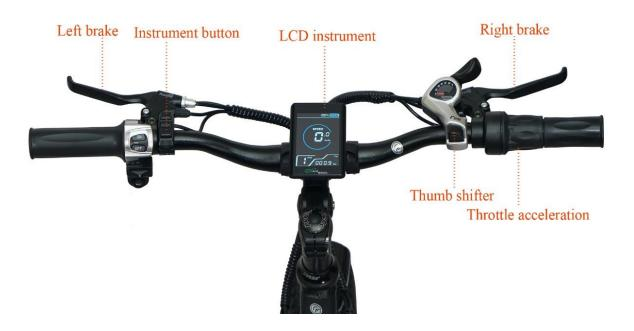
Long press(1 second) **Power Button** when the display is off, display, the display is fully displayed and starts to work, the power of the controller is turned on; Long press(1 second) **Power Button** when the display is on, display power off, the power of the controller is turned off. If you ride for 5 minutes (time can be set by the user) without operating the meter, the meter will automatically turn off the power.
