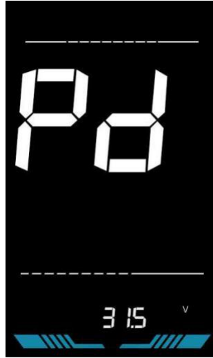
Figure 6-13 Battery under voltage value setting interface
