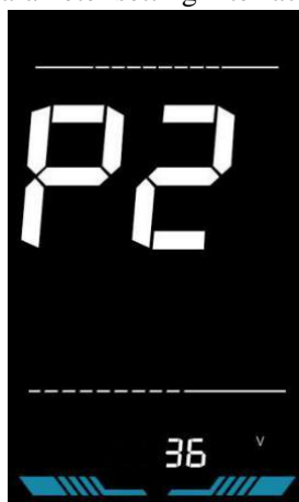
Figure 6-2 Rated voltage setting interface
